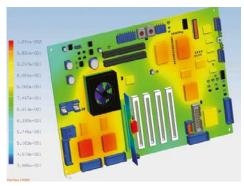
Simulation capabilities include thermal and flow analysis.
